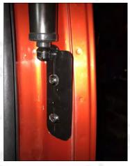
5.Remove the right lower bracket of the original car, install our left lower brackt and fixed it with our special screws.
