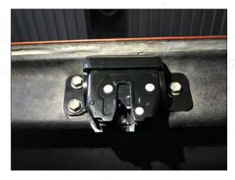
12.Unplug the original socket and plug in our front switch cable and reversing cable.
