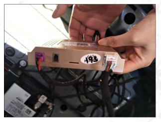
15. According to the color of the plug, insert the plug into the control box, and use our 3M paster on the back of the control box.
