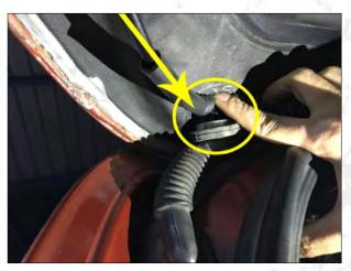
6.Remove the original car waterproof rubber plug, the cable passes through the rubber plug.
