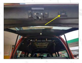
18. Punch the hole next to the tailgate electric suction lock, and then install our tailgate switch button.
