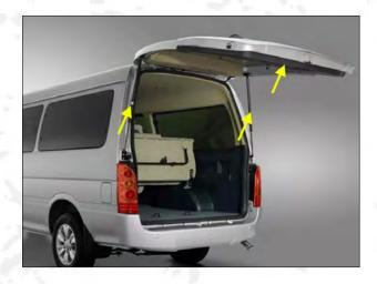
1.Remove the original car trim panel and brace rod.
