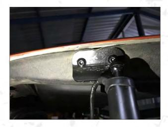
2.Remove the left upper bracket and the brace rod of the original car, install our brackets and brace rods (the ball head towards out) and fixed with our special screws.
