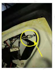
10. Find the screws inside the circle at the tailgate and connect it with our ground wire.
