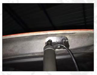
Remove the right upper bracket and the brace rod of the original car, install our brackets and brace rods (the ball head towards out) and fixed with our special screws.
