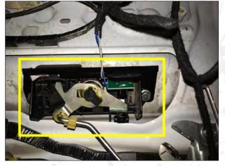
11.Remove the original car screws, install our brackets and fix them with the original car screws.
