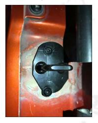
14. Remove the original car lock and install our lock.
