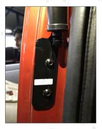
3.Remove the left lower bracket of the original car, install our left lower brackt and fixed it with our special screws.
